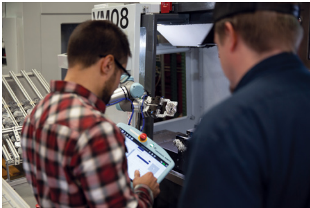
Troy Ojalehto (left) at Rapid Design Solutions, a Certified Systems Integrator of Universal Robots, developed the initial machine tending application with UR cobots at Toolcraft. The Seattle-based machine shop's automation engineer, Brian Laulainen (right), was able to handle the daily operation in addition to developing a parts rinsing and drying station as an application add-on for the UR5e. Laulainen did the training through the UR Academy, then supplemented with a few hours hands-on training with Ojalehto.
